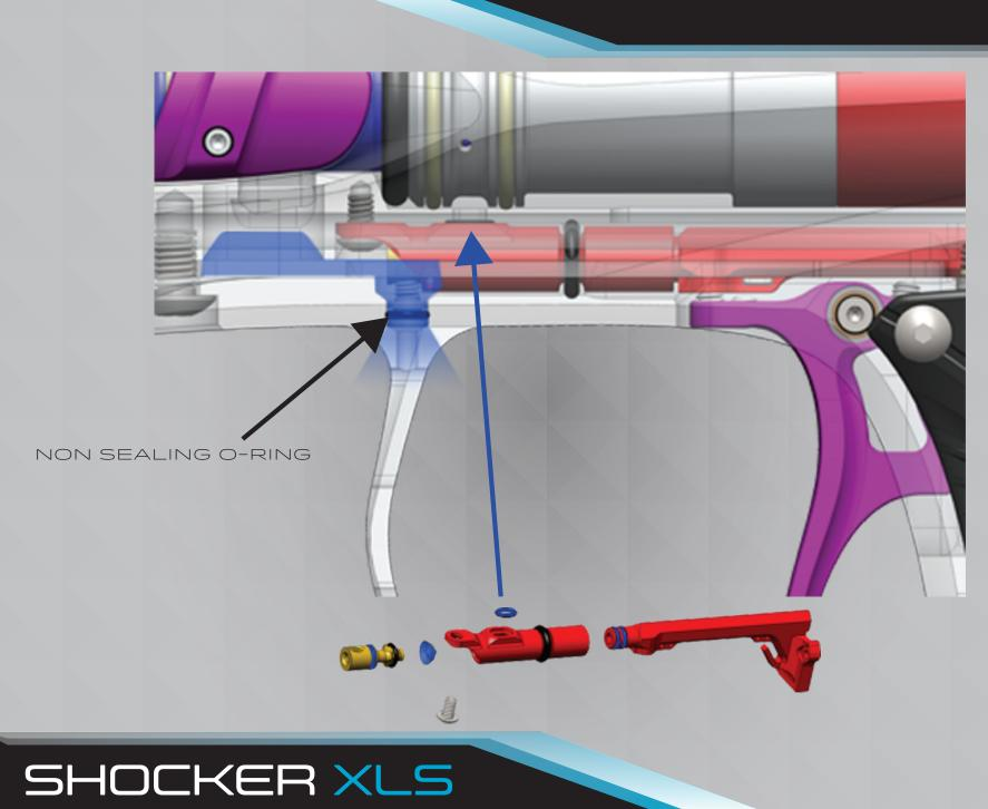
FORWARD FRAME LEAK GUIDE
