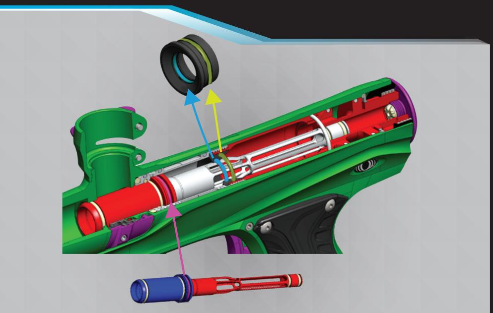
THIS DIAGRAM ILLUSTRATES THE O-RINGS RESPONSIBLE FOR AIR LEAKING FROM INSIDE THE FACE OF THE BOLT.
